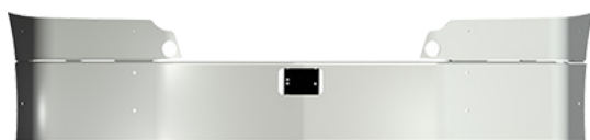
IU-0010-708-V10 Radar Cutout
